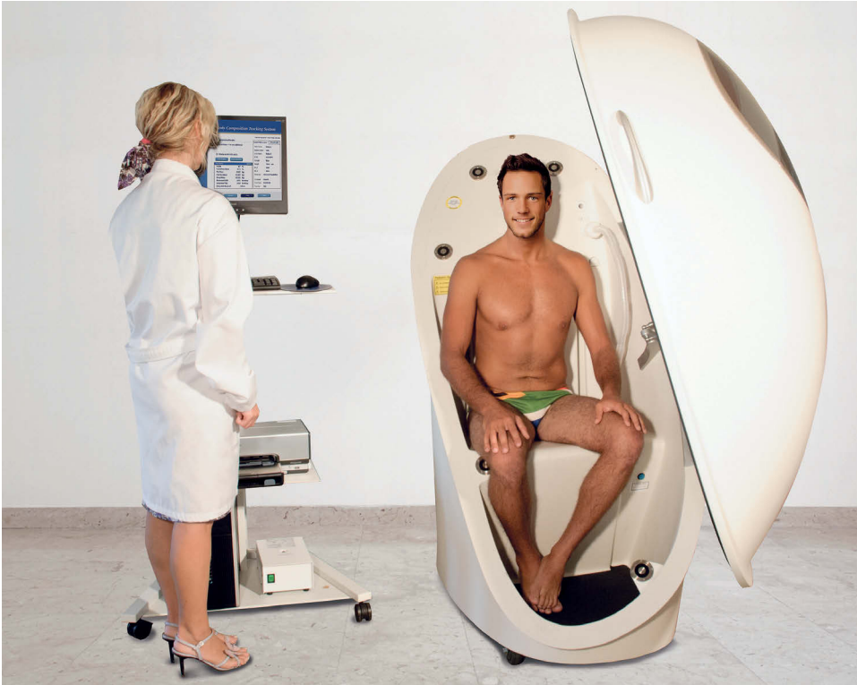
Cosmed's Bod Pod Gold Standard is a body composition (fat and fat-free mass) tracking system that uses whole body densitometry.
