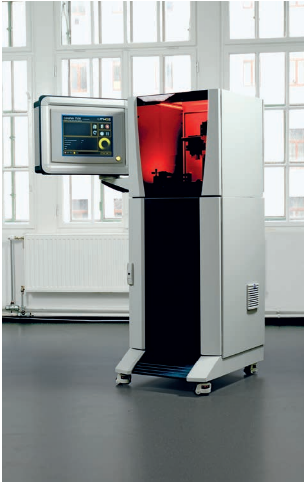
CeraFab 7500: Additive Manufacturing System for Ceramics.
