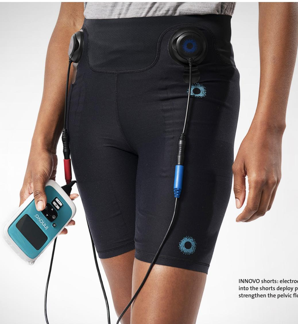
INNOVO shorts: electrodes integrated into the shorts deploy pulses to strengthen the pelvic floor muscles.
